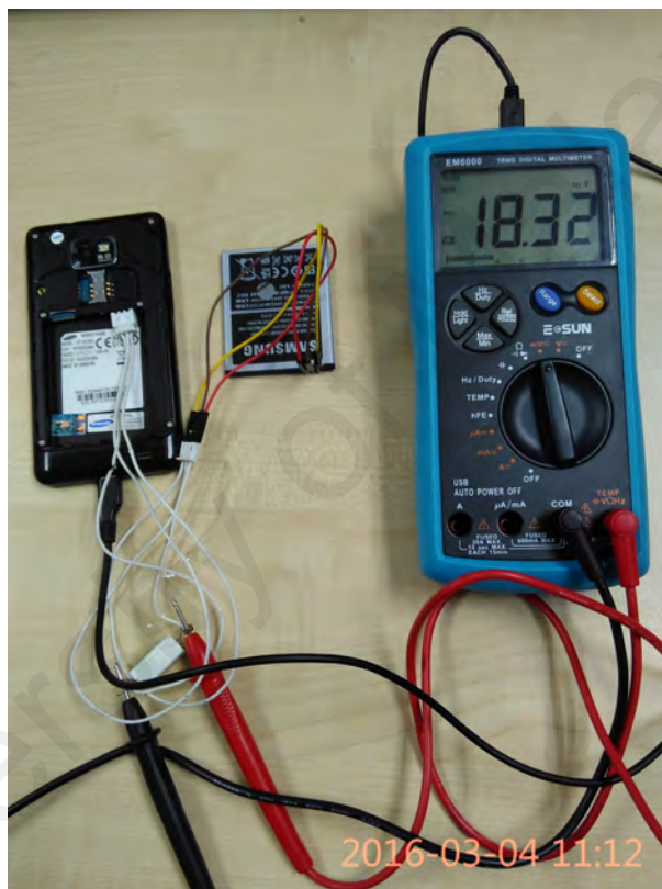
Figure 5.3: Experimental Setup for ARM-IS Energy Profiling
