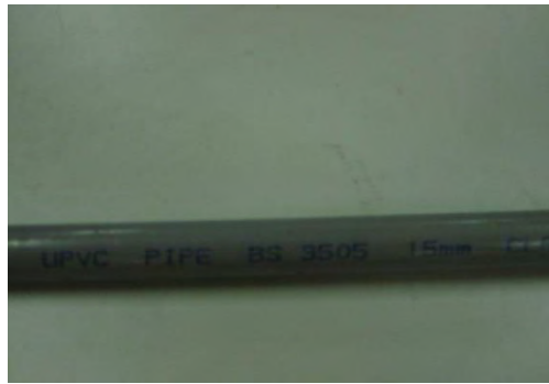
Figure 3.5: Photograph of the UPVC pipe used for the flow of the HTF.
