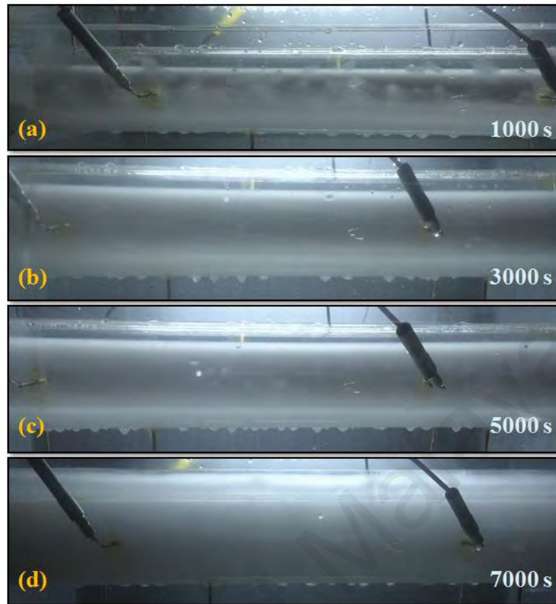
Figure 4.18: Solidification Process for distill water at Re=1000 and T_i= 30^\circ\text{C} in tube #1 at (a) 1000s, (b) 3000s, (c) 5000s and (d) 7000s.
