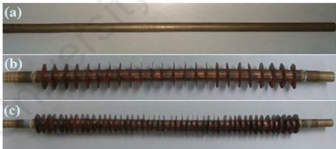
Figure 3.8: (a) The tube I (without fin), (b) The tube II (24 finned) and (c) The tube III (48 finned).
