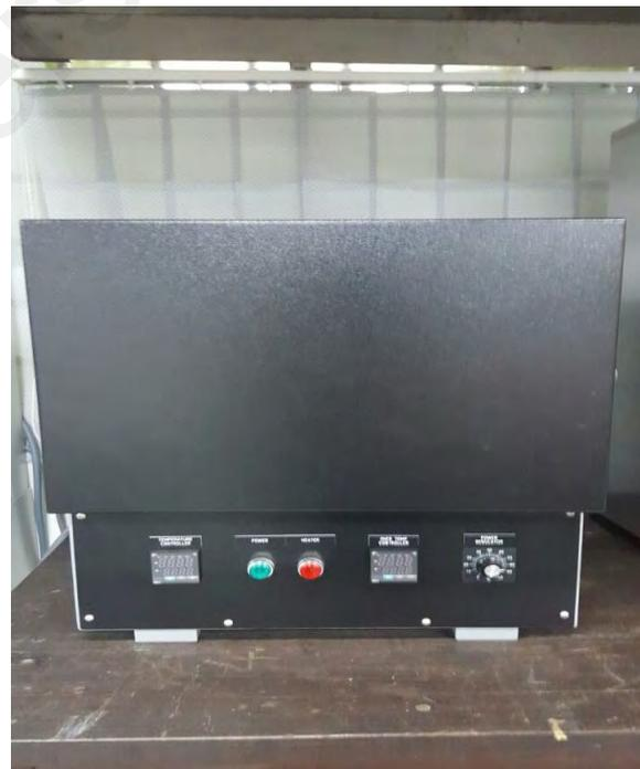
Figure B-2: Box Furnace used to perform conventional pressureless sintering
