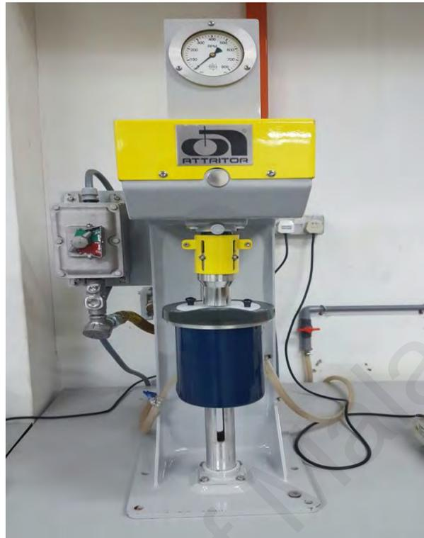
Figure B-1: Attritor Mill (Akron Electric Inc., USA) used to mixing calcined eggshell and calcium hydrogenphosphate dehydrate powder
