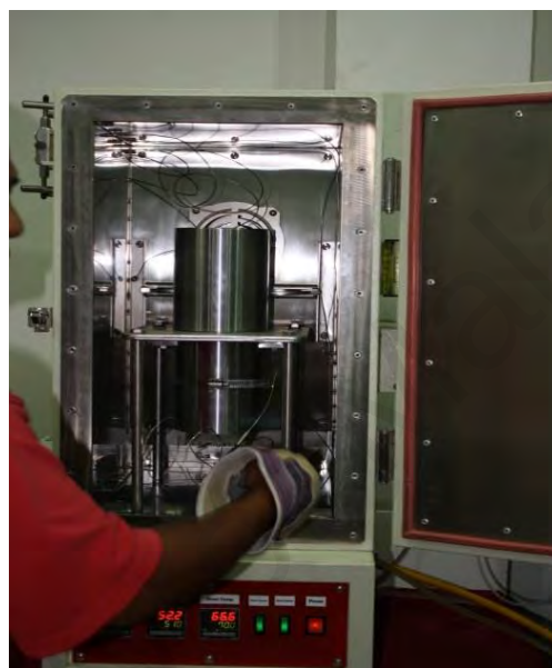
Figure 3-3: Oven Extraction Furnace
