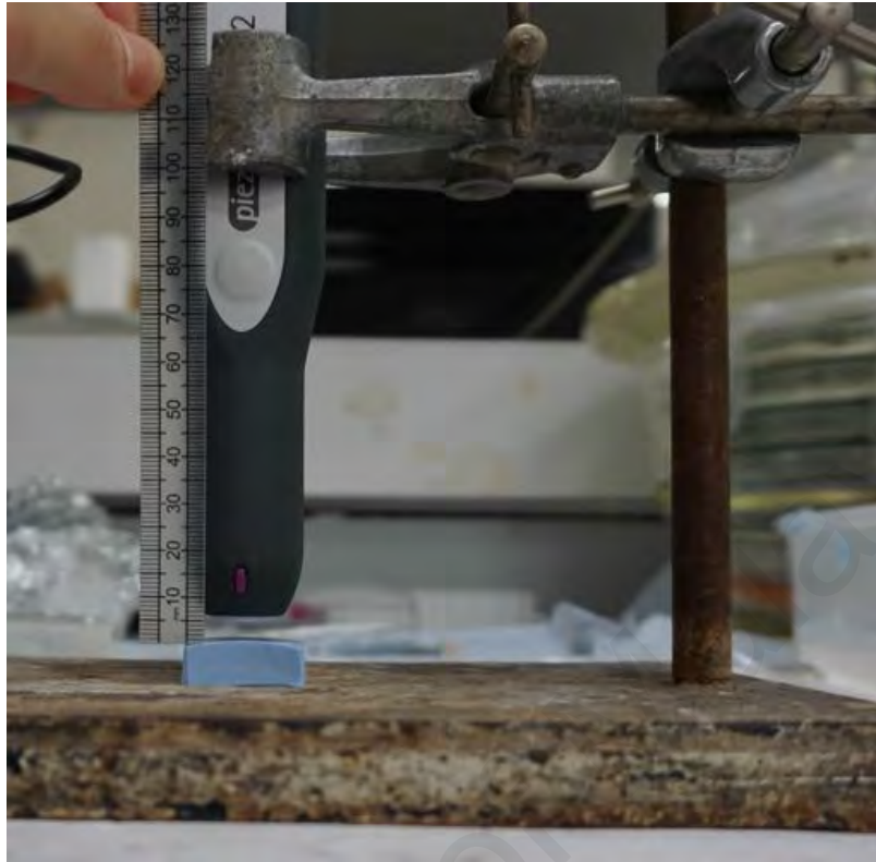
Figure 3: Non-thermal plasma device (Piezo Brush®PZ2 Handheld Device, Relyon Plasma, Regensburg, Germany) was fixed at a distance of 5mm from the adherend surface of zirconia.
