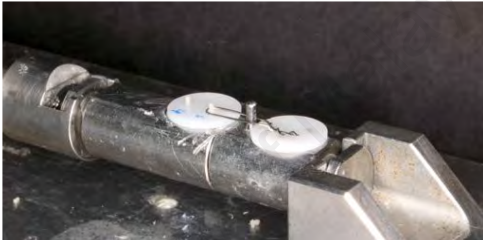
Figure 9: Specimens assembled and mounted onto a microshear bond strength test machine, ready to be tested.
