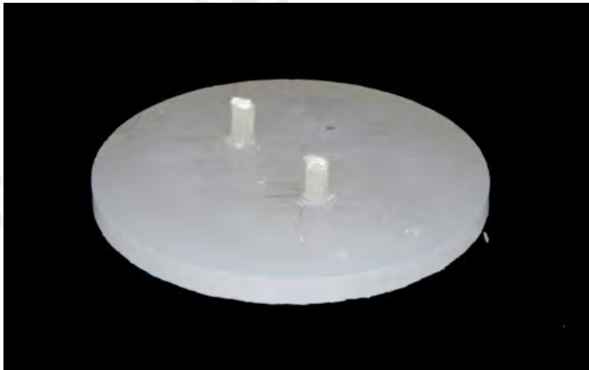
Figure 8: Resin cylinders bonded on zirconia surface after removal of Tygon tubing. Excess cement around the base of resin cylinders was then removed using a scalpel blade.
