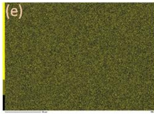
Figure 4.17: SEM images of \text{Bi}_{0.6}\text{FeCo}_3\text{Sb}_{12} skutterudite after 10 h BM and SPS, (a) micrograph of an SPS-compacted sample, an elemental mapping of (b), (c), (d) and (e) show Bi, Co, Fe and Sb by EDS.
