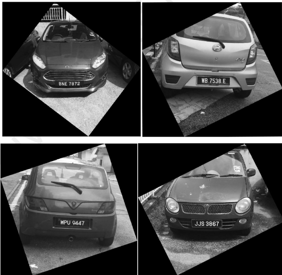
Figure 3.5: Vehicle images after skew correction
