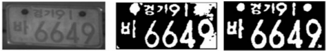
Figure 2.2: Plate images of noisy, after global and adaptive thresholding from left to right (B. R. Lee, Park, Kang, Kim, & Kim, 2004)
