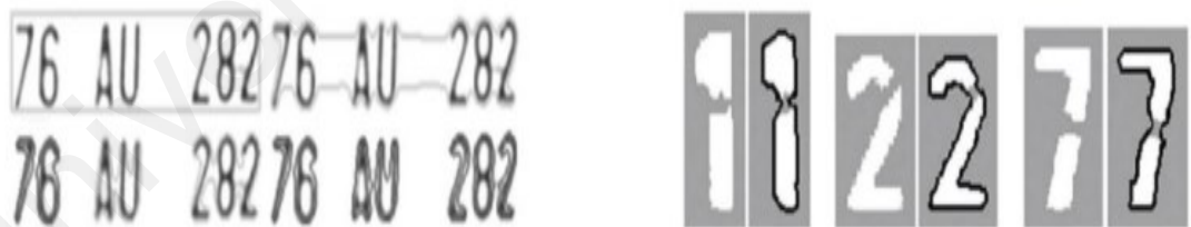
Figure 2.3: The sequence of segmentation & merging of the initially broken characters from left to right (C.-N. E. Anagnostopoulos et al., 2008)
