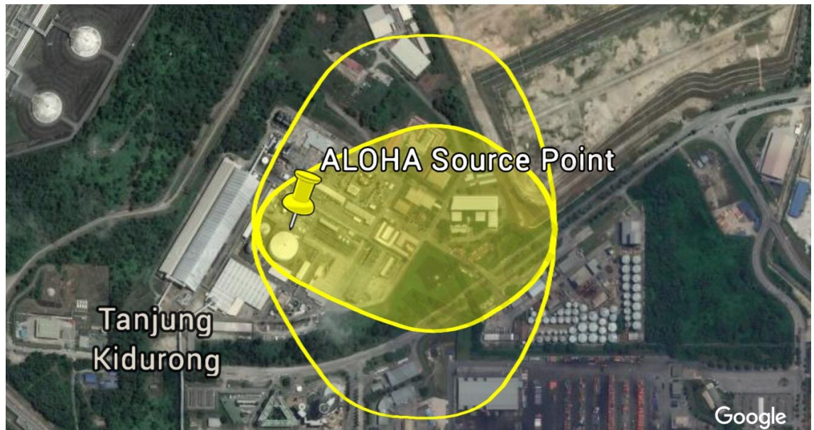
Figure 4.6 Impact of Overpressure from Ammonia Vapor Cloud Explosion
