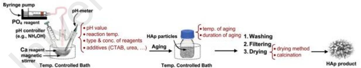
Figure 2.2: The synthesis process of HA via the wet chemical precipitation(WCP) route (Sadat-Shojai et al.,2013)
